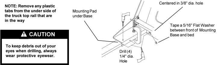
Step 4. Unclamp, Move Rack, Remove Flat Washer, Redrill Front Hole, and Install Blind Fastener
