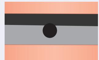
**Step 4:** The pilot hole is then aesthetically finished with a compatible material.
