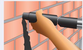
**Step 3:** Drive the Spira-Lok™ Wall Tie until the nose of the dry set installation tool is hard against the veneer.
