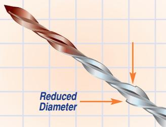
**Spira-Lok™ Asymmetrical Ties** are dual diameter **Spira-Lok™ Stainless Steel Helical Wall Ties** designed for use in connecting soft veneer materials to a hard back-up. Typically a larger installation pilot hole is required in hard substrates, such as concrete or brick, than, for example, in a soft veneer mortar.
