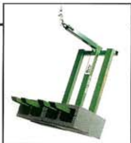
BLOCK FORK 800 lb. capacity 24 1 / 2 L x 24 1 / 2 W x 34 1 / 2 H For lifting 8 x 8 x 16 block
